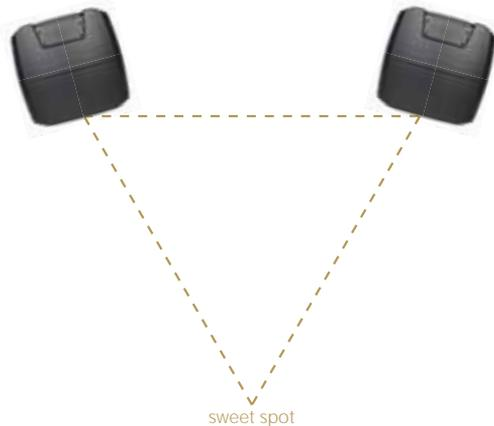
Mount the speakers slightly inward, so that the driver components directly face the listening position. When oriented this way, the listener is in the "sweet spot" which yields the most accurate stereo reproduction. If you need a wider sweet spot to allow for greater listener movement or for group monitoring, face the speakers in a slightly more open position, but never more than necessary.
