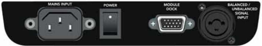
**Mains Input:** Connect the mains supply here. Ensure that you use only the cable supplied or a genuine EVENT replacement. Note that the amplifier is not entirely disconnected from mains power unless this cable is completely disconnected.
